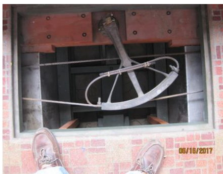
Steering Cable loose at Quadrant
