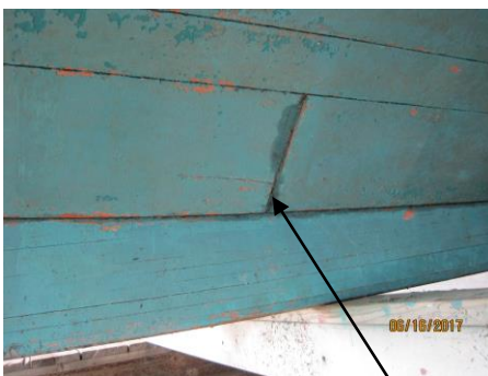
5 in. split in garboard – starboard
